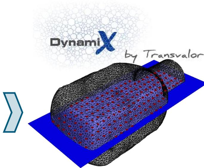
Strain and temperature evolution on a point grid
