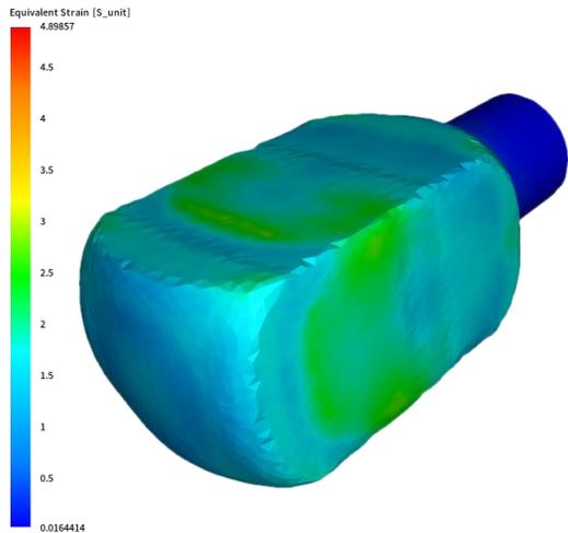
Strain and temperature evolution in the workpiece
