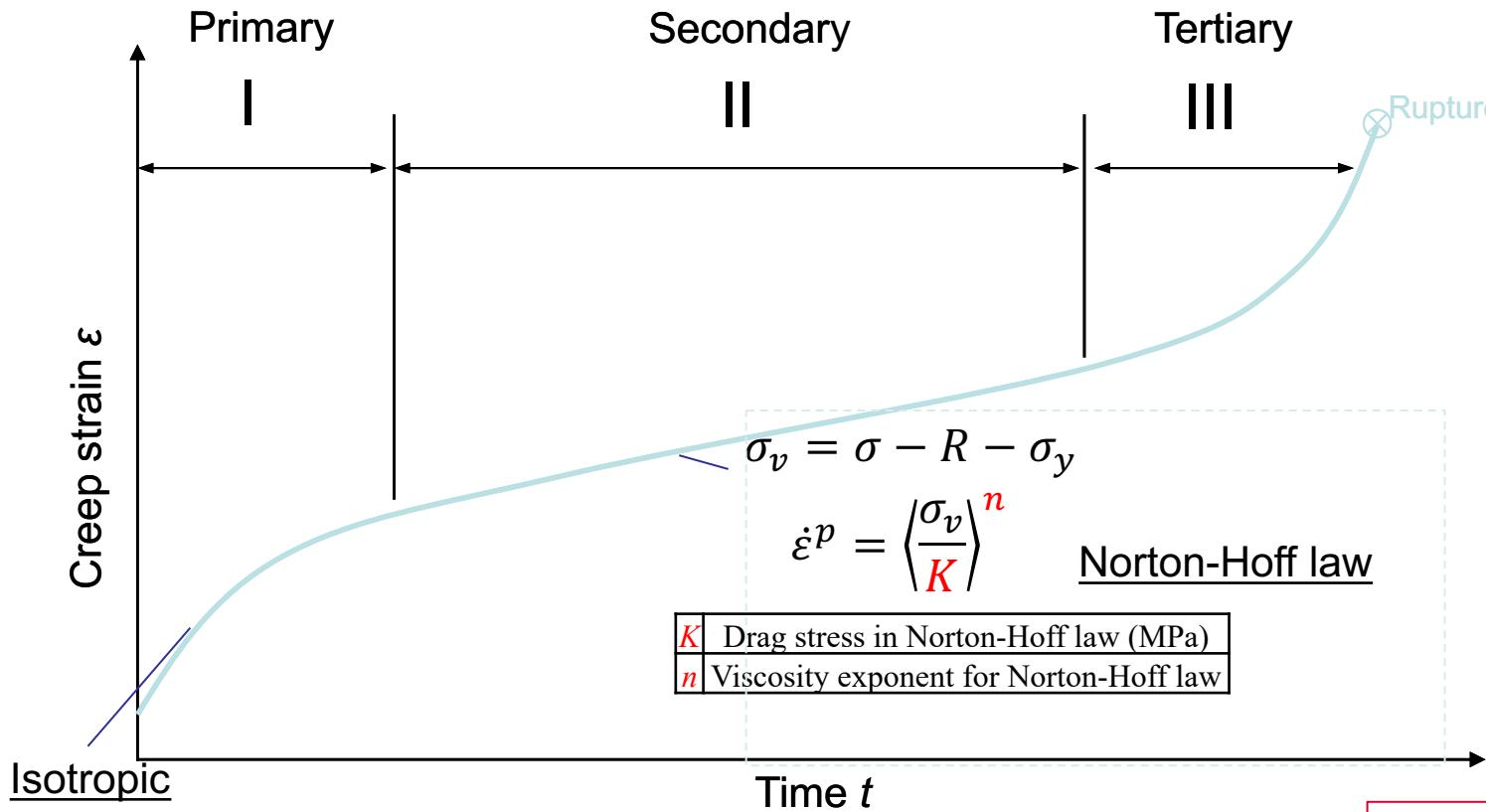
“Creep is a phenomenon of slow plastic deformation (elongation) of a metal at high temperature under a constant load.”
